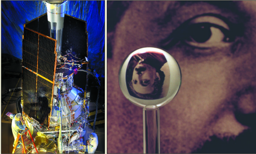
The Gravity Probe B (GP-B) satellite (left) is currently measuring two predictions of general relativity: frame-dragging and geodetic precession. The experiment involves detecting tiny changes in the motion of four gyroscopes that contain extremely smooth spheres made of fused quartz (right). The satellite, which is currently in a polar orbit at an altitude of 640 km, is a collaboration between Stanford University, Lockheed-Martin and NASA. The first results from GP-B are expected next year.
