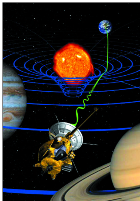
Right on time – an artist’s impression of the Cassini spacecraft flying between Jupiter and Saturn, and transmitting radio waves past the Sun and towards the Earth. The radio waves are delayed by their passage through the curved space–time near the Sun, an effect called the Shapiro time delay. Bruno Bertotti of the University of Pavia in Italy and colleagues have analysed these waves, and their value for the Shapiro time delay agrees with the predictions of general relativity to 1 part in 10^5 .
