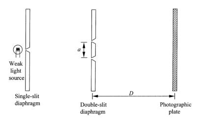
Figure 19.1. The two-slit experiment.
