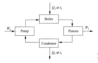
Figure 3.1. Diagram of the Woolf steam engine.
