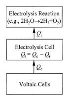
Figure 5.1. Input to and output from an electrolysis cell, according to Joule. The measured free heat  $Q_t$  in the cell depends only on the input  $Q_e$  from the voltaic cell and the output  $Q_r$  to the electrolysis reaction. It is equal to the input  $Q_e$  minus the output  $Q_r$ , that is,  $Q_t = Q_e - Q_r$ .
