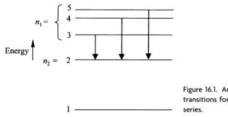
Figure 16.1. An energy-level diagram showing emission transitions for three of the lines in the hydrogen Balmer series.
