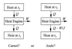
Figure 7.1. Heat engine operation between a high temperature  $t_2$  and a low temperature  $t_1$ , as viewed by Thomson in the conflicting theories of Carnot and Joule. Q represents heat, W work, J Joule's mechanical equivalent of heat, and  $\frac{W}{J}$  the heat equivalent to W. In the Carnot scheme, no heat is lost. In Joule's picture, an amount of heat  $\frac{W}{J}$  is lost.
