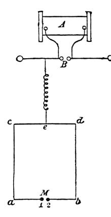
Figure 12.5. Hertz's coil circuit connected to a wire loop with a spark gap.
