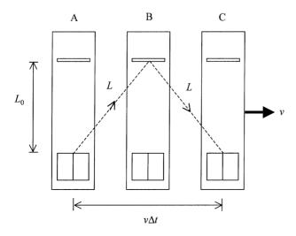
Figure 14.2. Einstein's light clock as seen by an observer who observes the clock moving at constant speed v.
