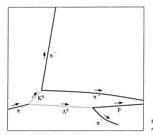
Figure 26.2. Interpretation of fig. 26.1. Only the relevant tracks are shown.
