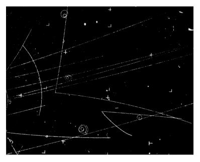
Figure 26.1. Photograph of tracks induced in a hydrogen-filled bubble chamber by a beam of high-energy, negatively charged pions. This photograph is reproduced by permission from the Lawrence Berkeley National Laboratory.
