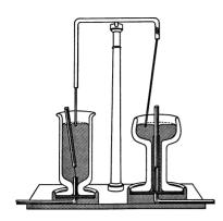
Figure 11.1. Faraday's experiments demonstrating electromagnetic rotation. From plate IV of Michael Faraday, *Experimental Researches in Electricity* (London: Taylor and Francis, 1839), vol. 2.
